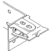
**NOTE:** Use the same holes for all brackets to ensure even projection from the surface.
